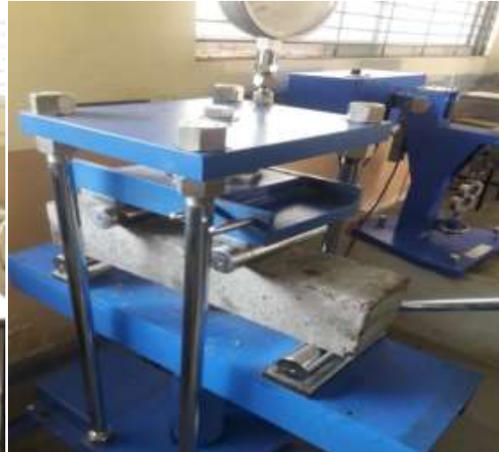
Figure No. 2:- Flexural Strength Test
